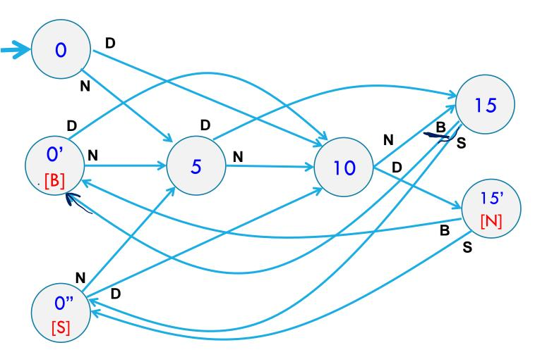
Adding output to states: N – Nickel, S – Snickers, B – Butterfinger
