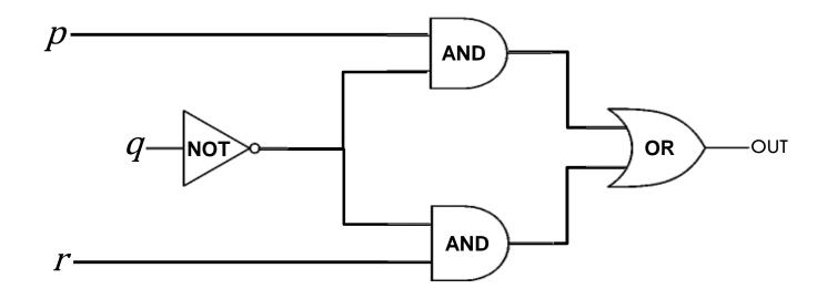
Wires can send one value to multiple gates!
