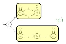
The top machine accepts strings with an even number of 1's The bottom machine accepts strings with the substring 11.
