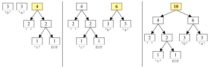
Notice that the nodes with low frequencies end up far down in the tree, and nodes with high frequencies end up near the root of the tree. This structure can be used to create an efficient encoding. The Huffman code is derived from this tree by thinking of each left branch as a bit value of 0 and each right branch as a bit value of 1:
