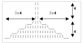
Please note that the height of the needle's midsection grows as the square of the figure size. In the default figure size of 4, the midsection is 16 lines tall. If the size were 7, the midsection would be 49 lines tall.
